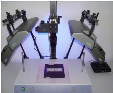
Fig.: Foto Light Box with RB5003 UV illumination
