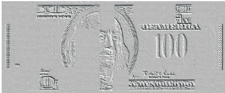
Lay-out of magnetic design on a 100-dollar banknote: in the emission of 1988-at the upper part, in the emission of 1996-at the bottom part.
