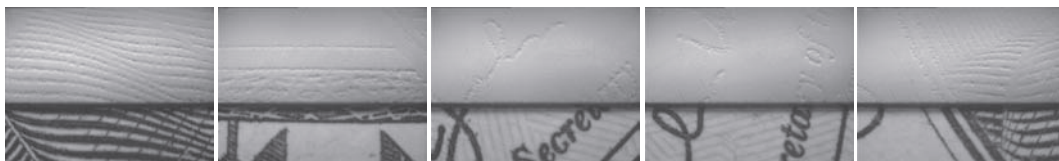
Magnetic-optical visualization of a 50-dollar banknote.
