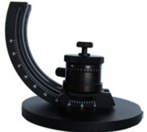
Bullet and cartridge case analysis stand with the movable pincers removed
