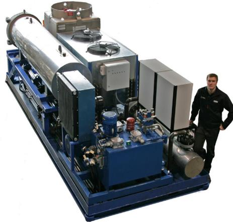
This manufacturing technology is ideally suited to the manufacture of high-quality, void-free, precision structural carbon fibre composite components for the aerospace and aviation industries. The XTclave™ CCT makes it possible to manufacture lighter, stronger and stiffer composite articles since the high magnitude of isostatic pressure can generate a fully dense composite with higher fibre content (better than 75%) for thermosets.
